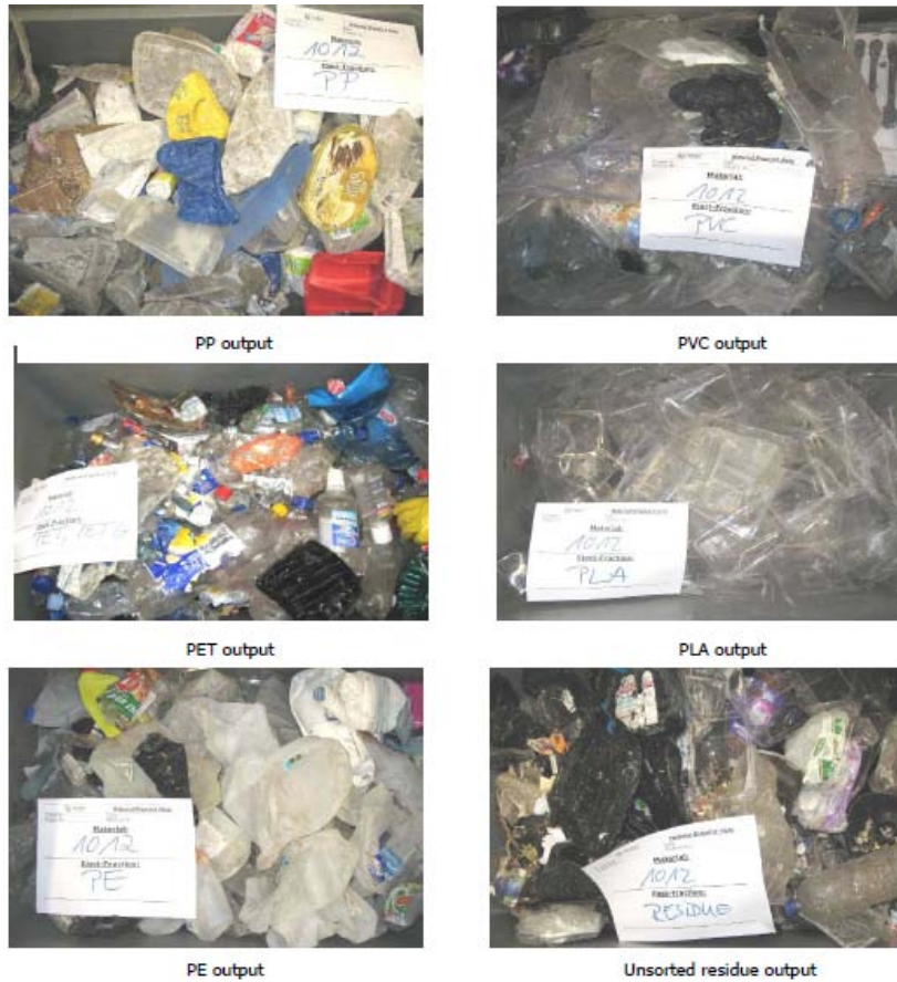
Figure 7. Successful Separation of Mixed Plastics Waste Stream (both rigid and flexible) Using NIR and Stadler Technology
