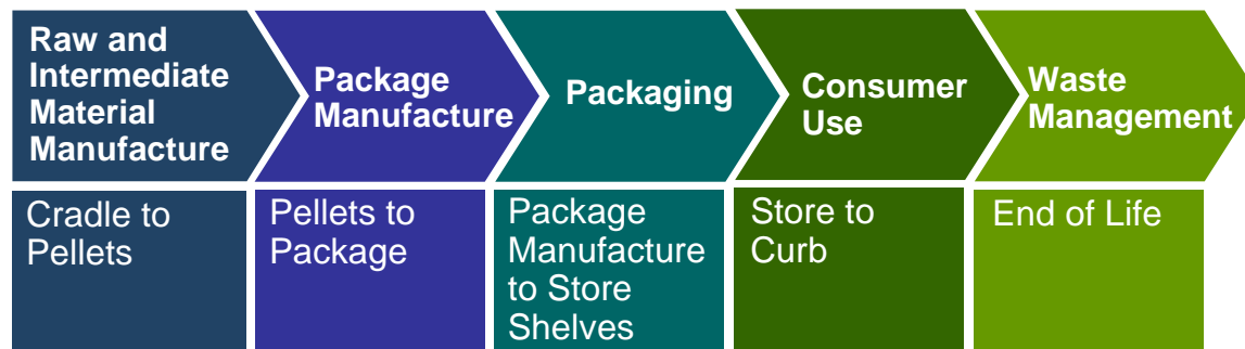
Figure 1. Example System and Life Cycle Stage Boundary Definition.
