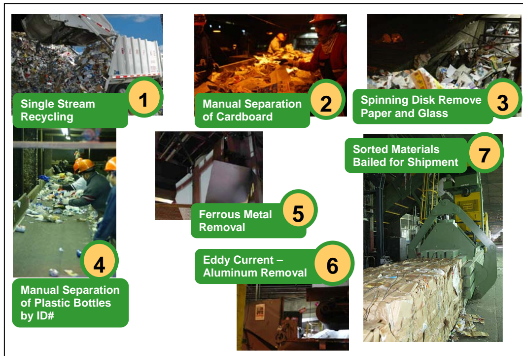
Figure 5. Single Stream Recycling of Residential Materials. 5
